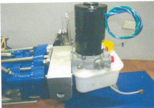
Cable Mount For Right Hand Drive with Pump Fitted
