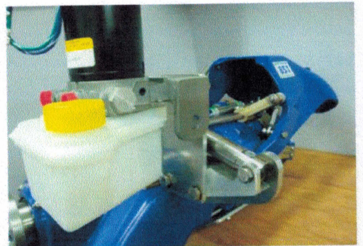
Cable Mount For Left Hand Drive with Pump Fitted
