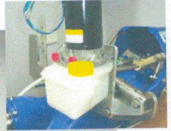
Reverse Pump Fitted Without Steering Mount
